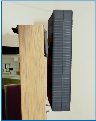
Models PEL 102 and PEL 103 can be mounted on a door or other object using the MultiFix mounting attachment, included.
