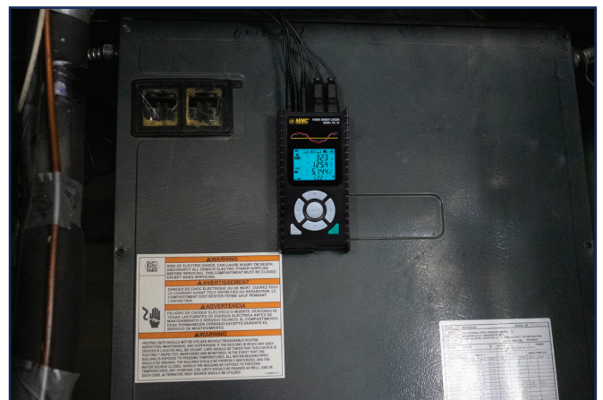
In this study, the load analysis was conducted using the AEMC® Instruments PEL 52. To secure the device in place during the week-long testing period, two powerful magnets on the casing allow it to be easily attached to the flat metallic surface of the HVAC system.
